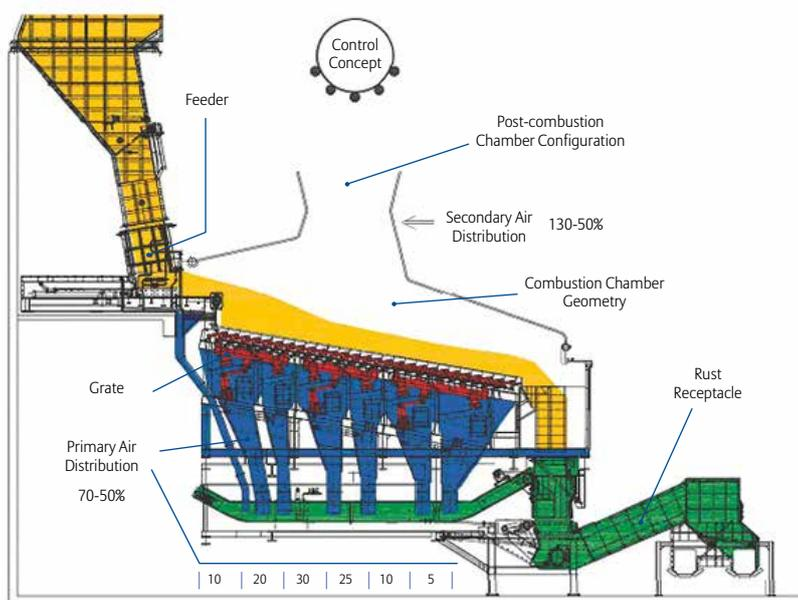
Figure 1: Stoker-fired furnace in detail.
