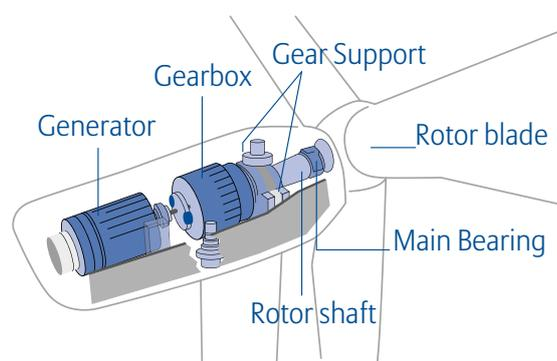
Figure 3: Three-point support of the rotor shaft
