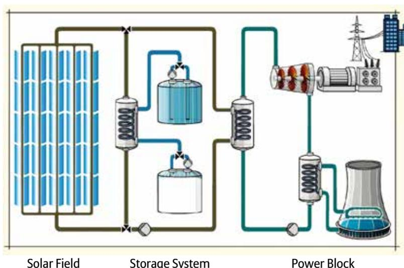
Figure 1: Components of a parabolic trough power plant
