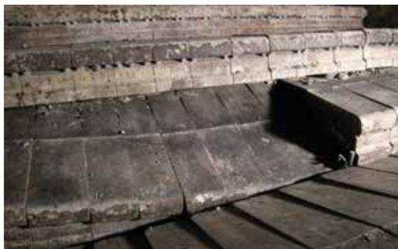
Figure 2: Damage of the grate as a result of overheating and corrosion
