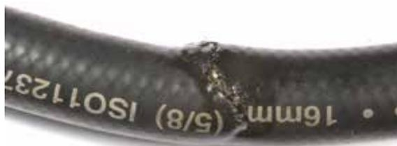
Image 5: Burst hydraulic hose line with a leak formation.
