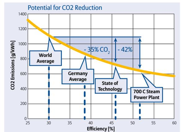
Figure 1: Development of potential CO<sub>2</sub> reduction/efficiency. (Source: BMWi, Turbomachinery 2006)
