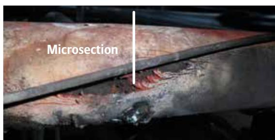
Figure 4 & 5: Split area (left) and trace heating line above the breakage area (right).
