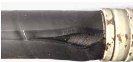
Image 1: Damaged hydraulic hose line
