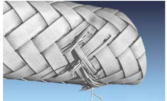
Image 6: CT scanning of the area of the leak, from Image 5. The dent in the area of the leak indicates that the hose was clamped and damaged.
