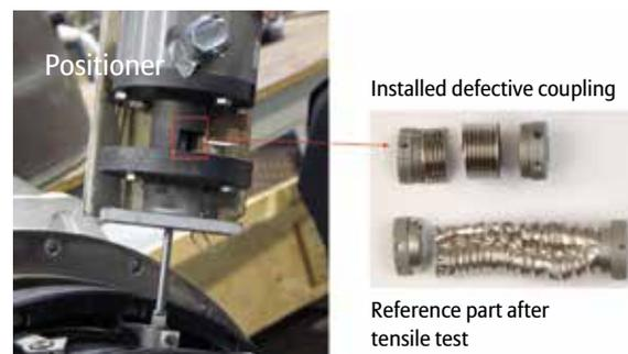
Figure 4: Broken coupling piece
