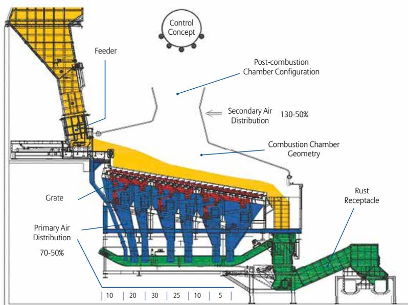
Figure 1: Stoker-fired furnace in detail.
