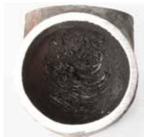
Figure 6: Deposits on the pipe interior.
