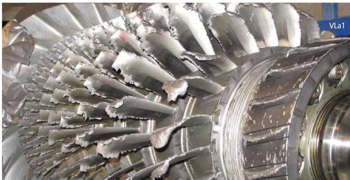
Figure 3: Compressor damage (image: AZT).
