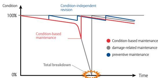
Figure 6: Comparison of the different maintenance concepts.
