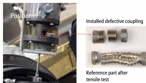
Figure 4: Broken coupling piece
