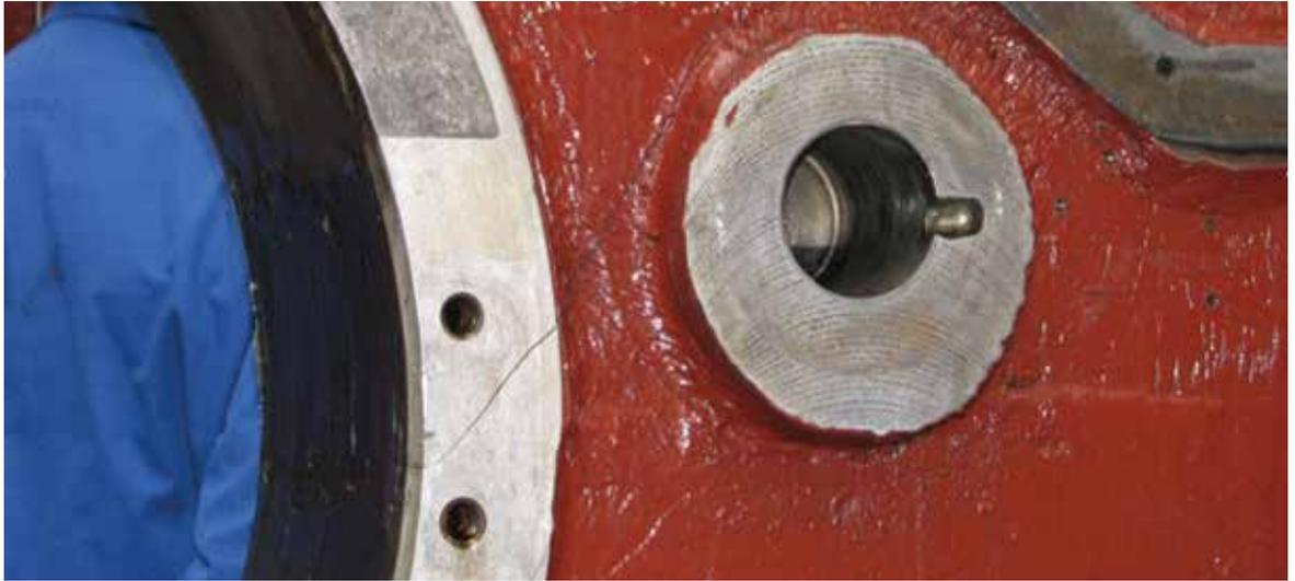
Figure 1: Crack in the frame of a progressive press
