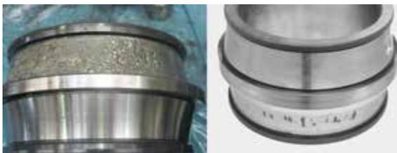
Figure 4 & 5: Damaged spherical roller bearings – planetary bearings (left) and damaged spherical roller bearings – rotor bearings (right).
