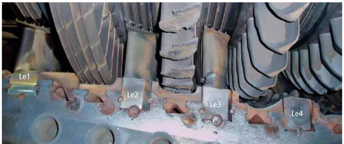
Figure 2: Damage pattern in the high-pressure turbine (image: AZT).
