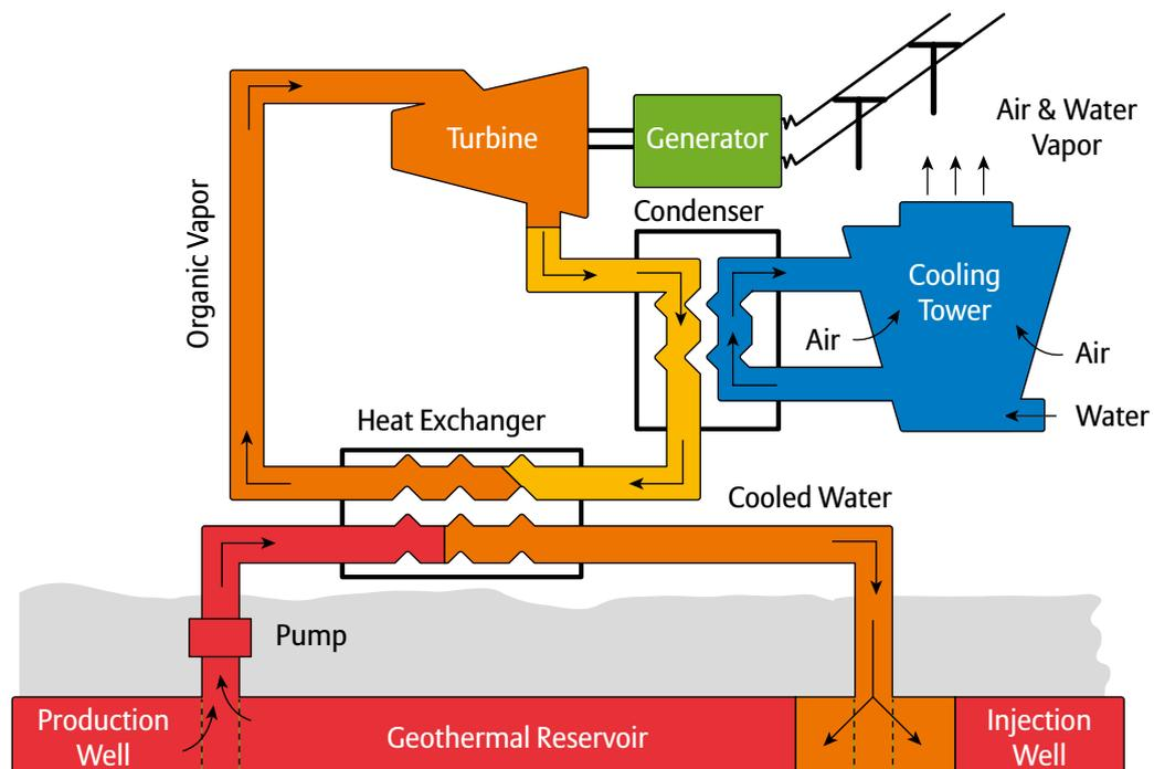
Figure 1: A geothermal power plant in detail.
