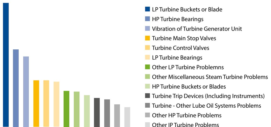
Figure 1: Loss of availability from different causes of damage (relative comparison) (Source: EPRI/NERC)
