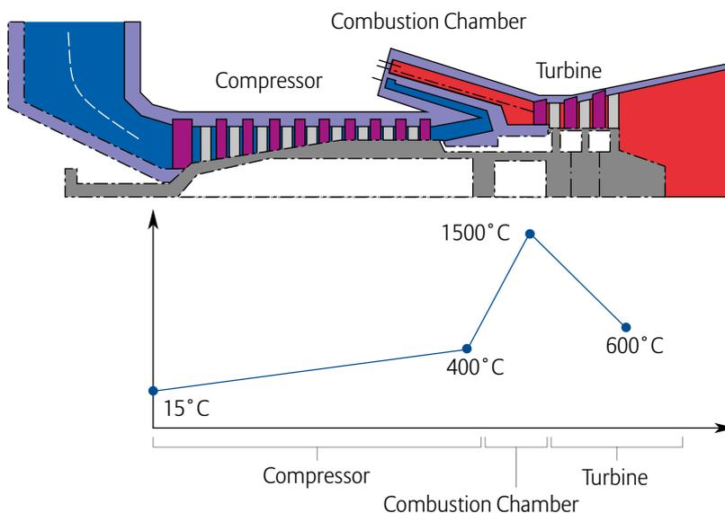
Figure 1b: Component temperature profiles
