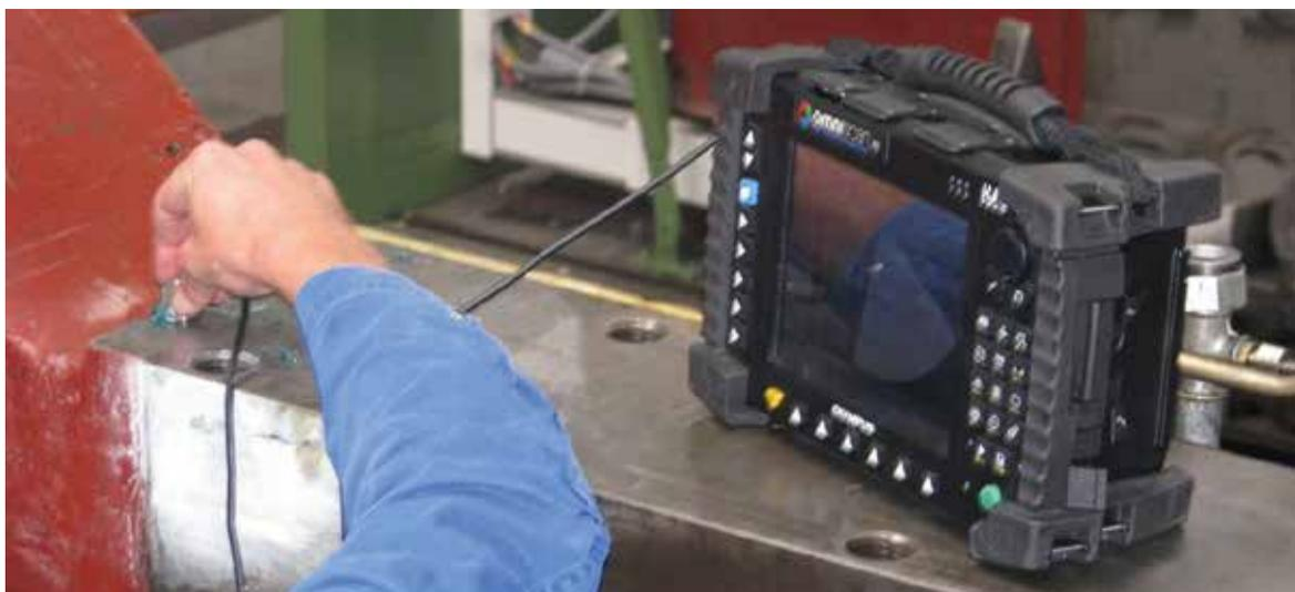
Figure 2: Phased Array Ultrasound Test (PAUT) of the area surrounding the crack
