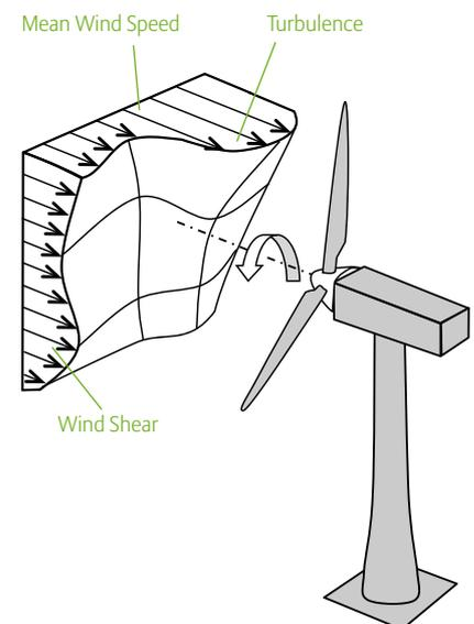
Figure 1: Schematic wind field pattern
