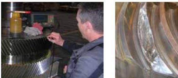
Figure 1 & 2: Tooth volume testing and gearing damages
