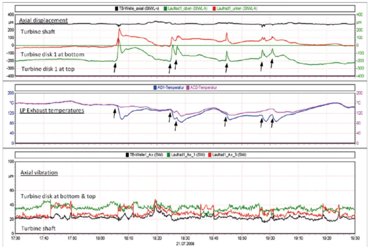
Figure 2: Vibration progressions showing various results from the introduction of water (indicated by arrows).
