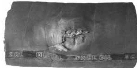
Image 4: The linear impression on the surface of the hose indicates a hose which was trapped or crushed in the area where the damage occurred.
