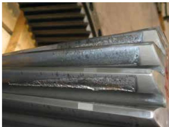
Figure 2: Sun pinion with tooth flank damages resulting from an irregular load distribution.
