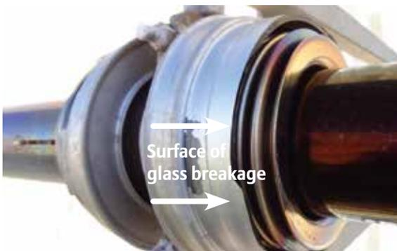
Figure 3: Typical glass breakage near the glass-to-metal seal.
