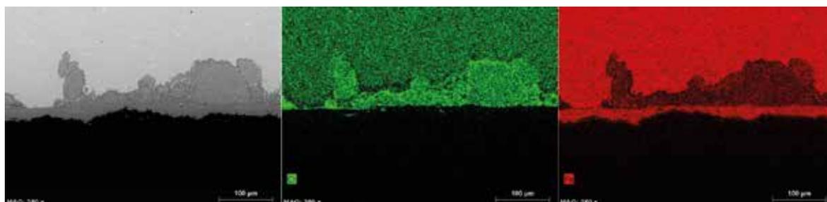
Figure 2: Example of an oxide layer of the 18Cr11NiNb material as seen through a scanning electron microscope (left), and the distribution of chrome (in green) and iron (in red).
