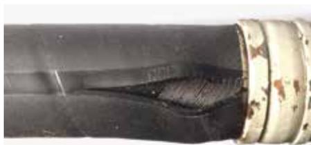
Image 1: Damaged hydraulic hose line
