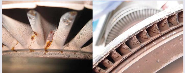
Corrosion in the gap of the blade grooves
