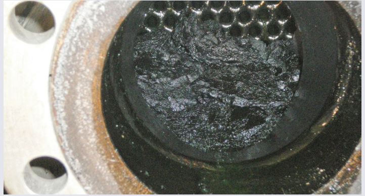
Carbonized oil in a heat exchanger of a thermal oil boiler
