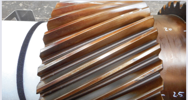
Varnish on flanks of a pinion shaft
