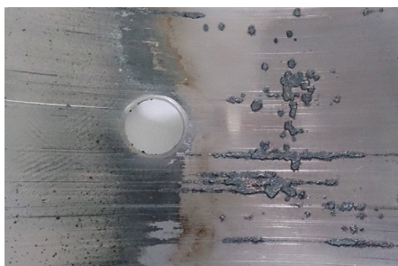
Selective corrosion in a gas motor plain bearing
