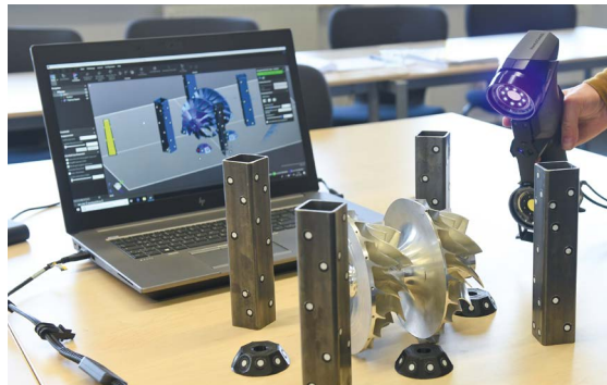
Fig. 2: 3D scan of investigated component
