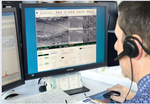
Fig.3: Analysis in the scanning electron microscope a) and transmitted via web meeting to the engineer/client b)
